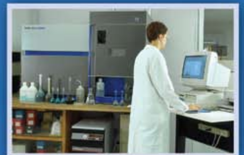
ICP determines the type and amount of elements in samples
