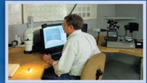
Digital imaging system magnifies to 1000X
