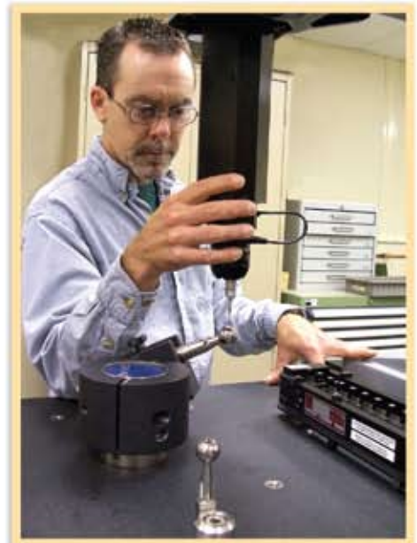
CMM calibration with a ball bar and step gauge
