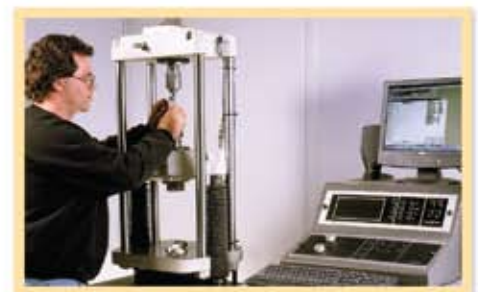
Tensile testing on 60,000 lb. capacity machine
