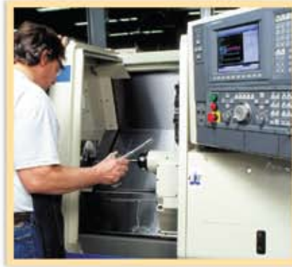
CNC turning center cuts cylindrical specimens for testing
