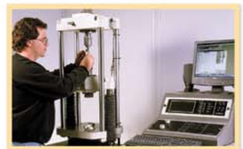
Tensile testing on 60,000 lb. capacity machine
