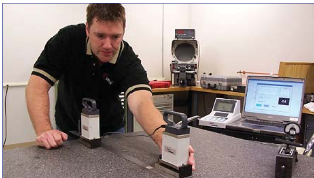
Computerized surface plate calibration using leveling feet
