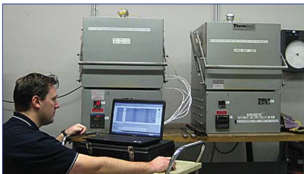
Conducting an oven survey to meet Nadcap requirements for AMS2750D
