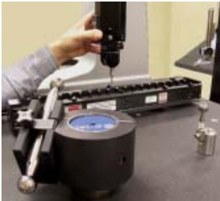
CMM calibration with ball bar & step gauge
