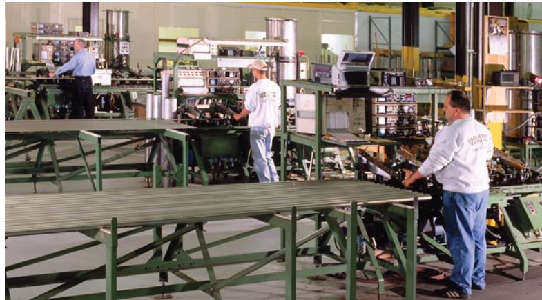
Three UT immersion systems for round materials up to 75 ft. long
