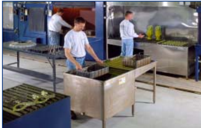
Fluorescent dye penetrant dip tanks, wash station & oven
