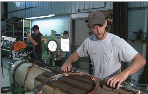
Hydrostatic Pressure Testing
