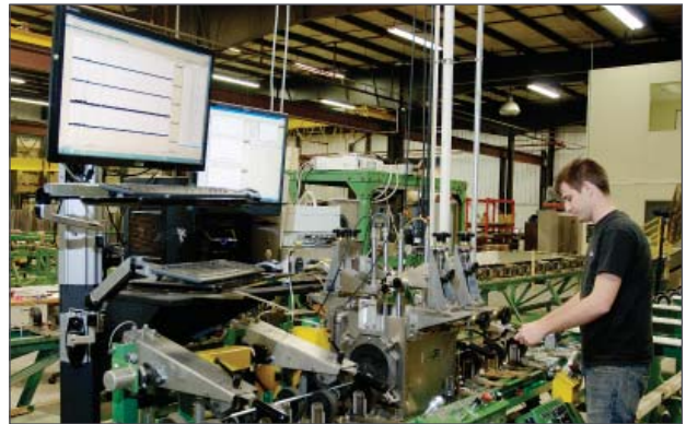
Immersion Ultrasonic Testing of tubing
