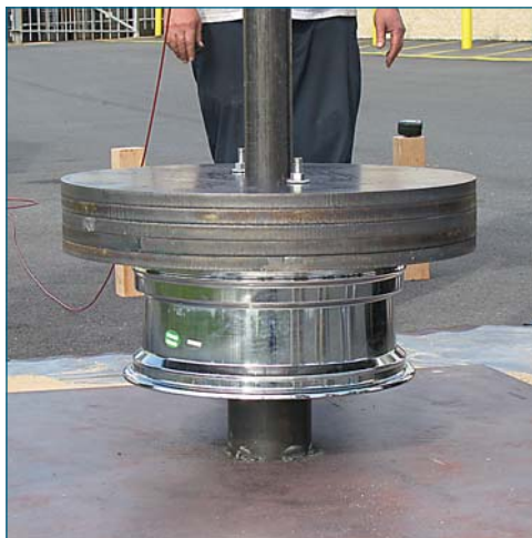
Drop-weight test conducted on one of two styles of tire rims.
