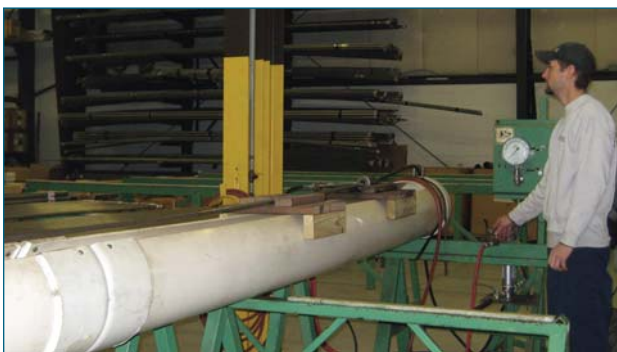
Hydrostatic Testing performed on copper/nickel tubing
