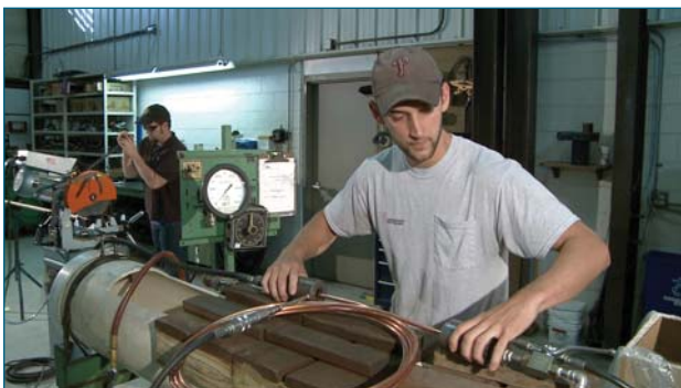
Technician prepares copper coil for Hydrostatic Testing
