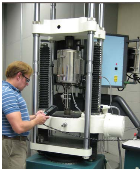
Elevated temperature furnace carousel behind new 120K tensile testing machine
