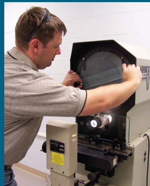
Field calibration of optical comparator
