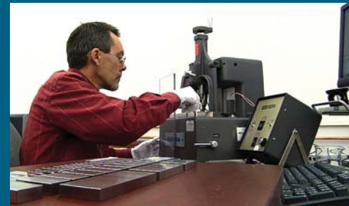
Gage block calibration
