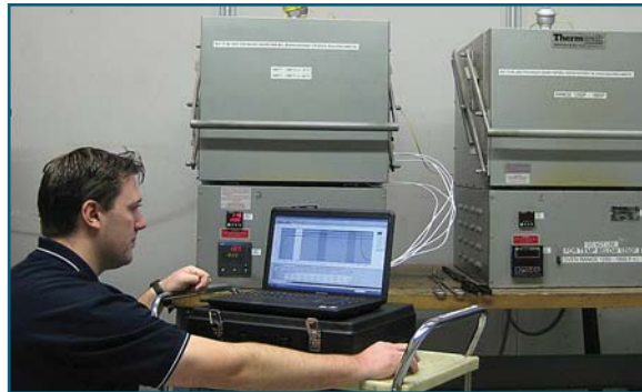
Conducting an Oven Survey to meet Nadcap requirements for AMS2750D
