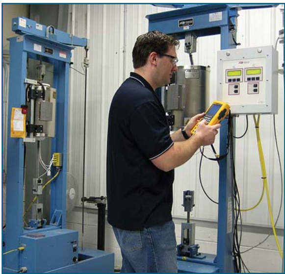
Calibrating a Temperature Controller for a stress rupture machine.
