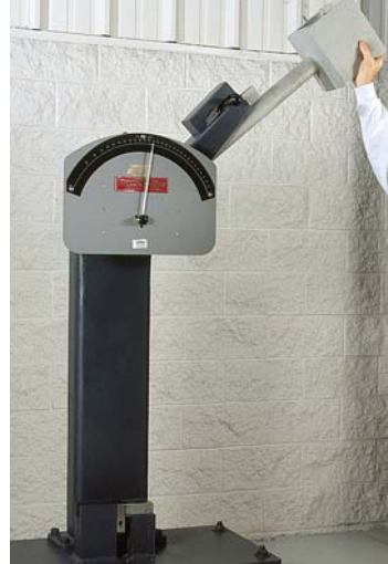
Pendulum ready to swing toward test specimen
