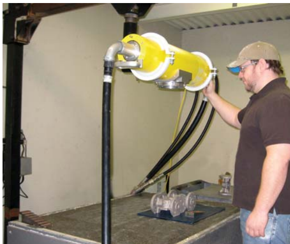
X-ray tube in 20 ft. x 20 ft. Radiography Vault
