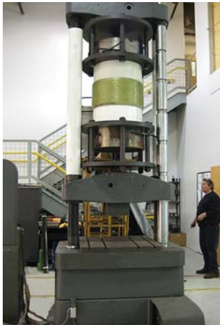
Well casing joint assembled for proof-load testing to destruction
