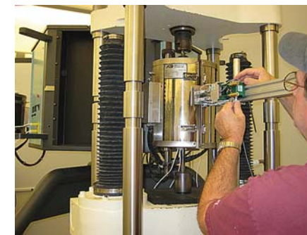
New extensometer measuring strain
