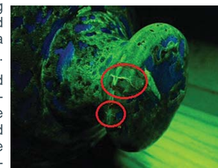
Noting cracks on the barrel knob
