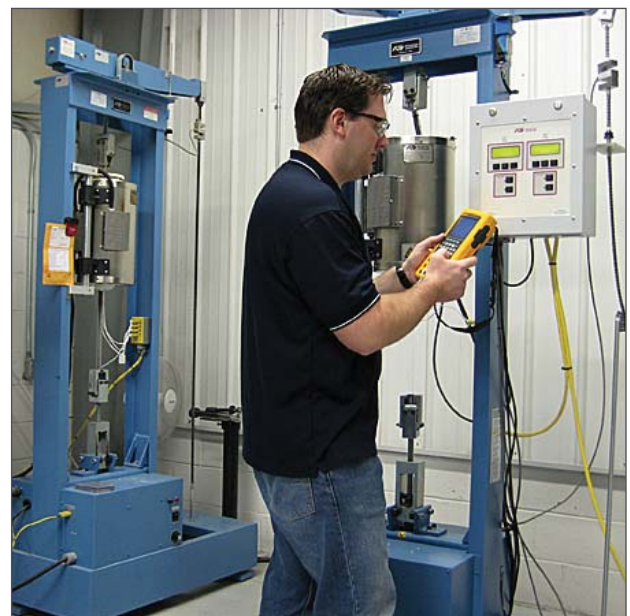
Calibrating temperature controllers on a stress rupture machine
