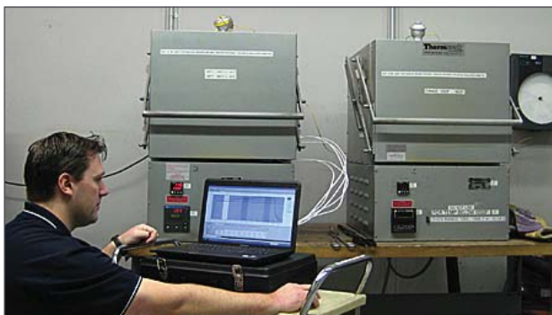
Conducting an oven survey to meet Nadcap requirements for AMS2750E
