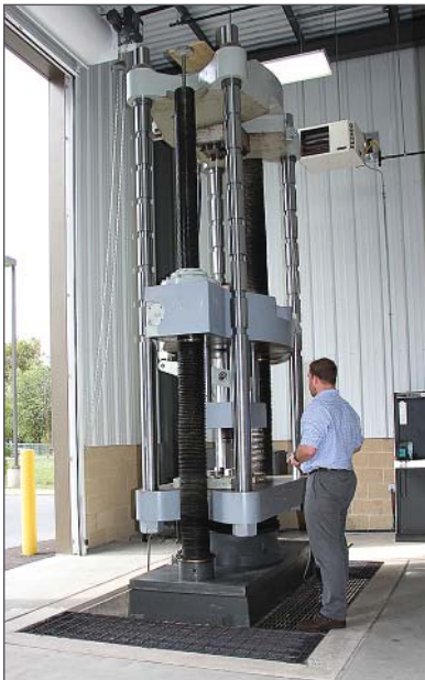
Tensile testing to 600,000 lbs.
