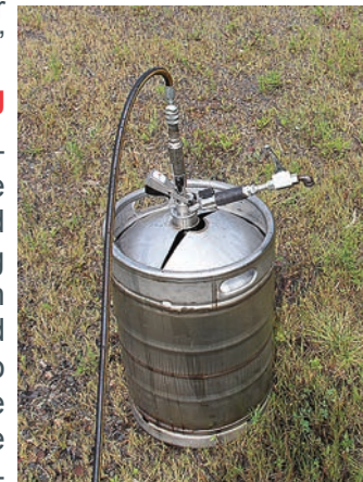
Burst along weld near tap
